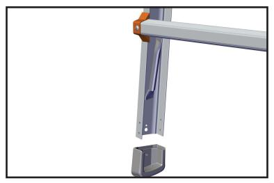
5. Place the new standard feet on the ends of the rails. The small hole in the feet should align with the small holes in the rail. Note: There are left and right feet. The pointed end of the foot goes to the outside of the ladder.
