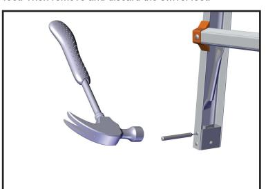
3. Using a hammer and 3/16" punch, completely remove the rivets securing the spacers.
