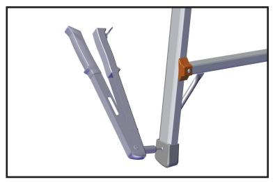
6. Insert pop rivets into the feet, and set with a rivet gun. Make sure all feet are set and ladder is secure before using ladder.
