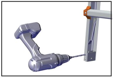
2. Using a drill with a 3/16" drill bit, remove the heads of the rivets securing the spacers. Use a hammer and chisel as necessary to completely remove the rivet heads.
