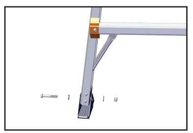
1. Using two 1/2" wrenches, remove and discard the existing nuts, bolts and washers securing the swivel feet. Then remove and discard the swivel feet.
